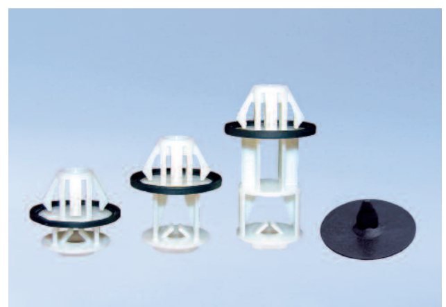
Dowel-type 2C floor trim retainers serve to hold down the lining on automotive longitudinal chassis beams. The actual fastener consists of polyamide. The non-hardening sealing ring moulded on to it is made of a styrene ethylene butadiene styrene (SEBS) and prevents an ingress of water and moisture.
