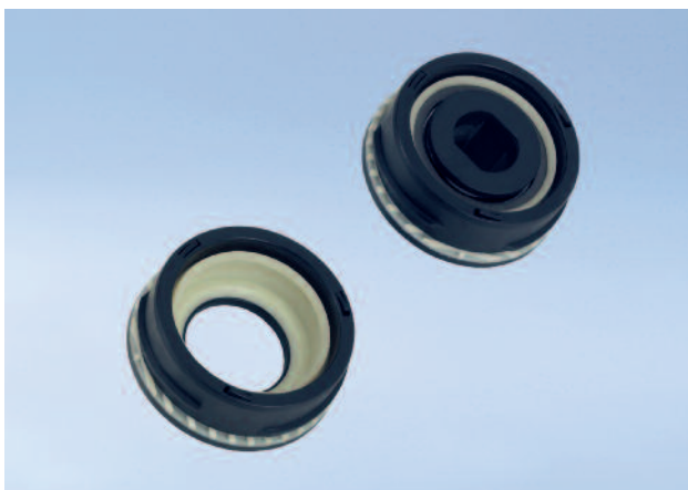
This 2C bearing insert provides additional support for the steering column while also holding back noise and acting as a seal against splash water and dirt. The ball bearing is held securely in the soft TPE component in a positive fit. The hard component snaps into a bearing housing upon assembly and remains inseparably joined to it.
